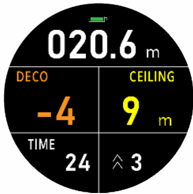
Scuba Mode – Underwater When the NDL has been exceeded (after three minutes)
