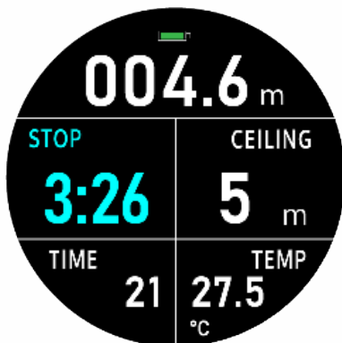
Scuba Mode – Safety stop (When the NDL has not been exceeded)
