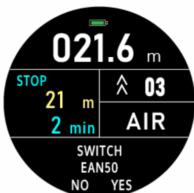
Tec Mode - Underwater Recommended Gas Switch
