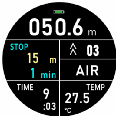
Tec Mode - Underwater When the NDL has been exceeded
