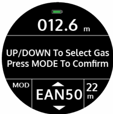
Tec Mode - Gas Switch (Switching)
