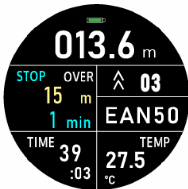
Tec Mode - Underwater When reaching the depth indicated for Decompression Stop but no Stops are performed
