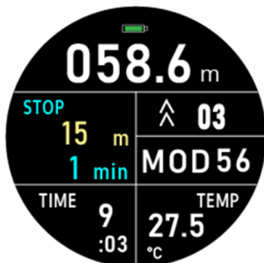
Tec Mode - Underwater When the MOD has been exceeded
