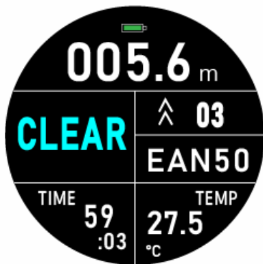
Tec Mode - Underwater When exceeding the NDL, and Decompression Stop at CEILING depth has ended.
